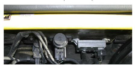
To test, go under the front of the car and remove the vacuum line from the Pulse air Injection system black box. Connect a vacuum gauge. You should get vacuum only on a cold engine and overrun. If there is any vacuum at idle on a hot engine then the solenoid is broken. Replacement is £25 and just the two screws hold it on. A very rough idle to stalling are the symptoms
