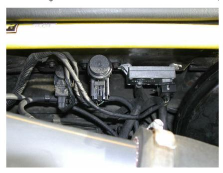
THE EGPD Valve is the silver box on the right. There are just the two screws holding it on. Also check the rubber vacuum lines running to it as they can split
