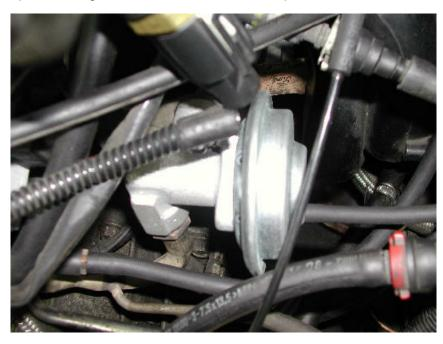
(Above) A shiny new EGR valve, note the vacuum hose running from the front of it. You can see the base of the Inlet Air Temp Sensor above it.
