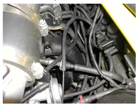
(above) The mass of vacuum and fuel lines behind the Zetec. Having removed all the plenum chambers makes this easy to see. In fact on my car the plenum chamber had chaffed several lines. EGR Valve and Inlet Air Temp sender
