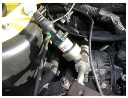
In my case you can see that I have replaced the wires and fitted a new rubber shield. My original wires broke at 30K miles.
