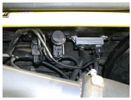
Its possible to clean it out using Throttle Body cleaner but it wont be that dirty. To test, remove the vacuum hose from the EGR valve and put a vacuum gauge on it. It should only show a vacuum at part load settings. If it shows vacuum at idle or wide open throttle then the solenoid is duff.
