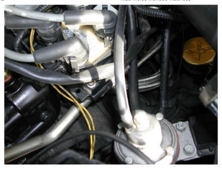
My Coil, the T piece connects the thick silver tube on the lower left to the thin tube to the right of the coil, and the third way goes to the engine block. It just pulls off
