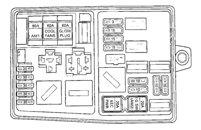
This box is easy to find. It is on the passenger side of the engine compartment at the front next to the Battery. Helpfully the lid inside is marked with all the fuses and relay information
