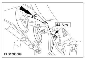
51. Bolt the torque converter onto the drive plate (four bolts).
