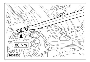
60. Attach the front axle transverse brace to the side member.
