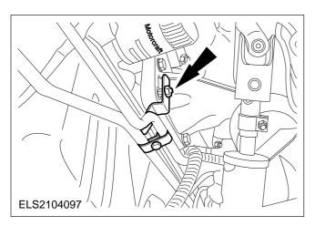
36. Unscrew the transmission flange bolts on the left-hand side.
