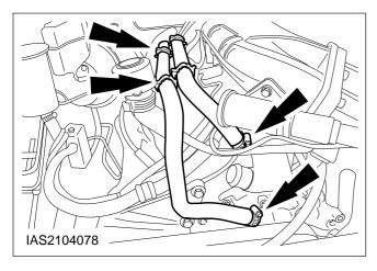
9. Disconnect the expansion tank connecting hose and the upper coolant hose from the thermostat housing.
