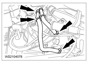
81. Fit the coolant hose for the heating on the thermostat housing and the coolant hose onto the coolant pump.
