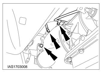
32. Disconnect the front left-hand exhaust pipe.
