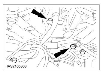
**39.** Remove the coolant pipe.
