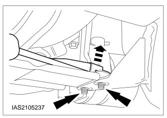
51. Detach the transverse brace from the front crossmember (left-hand side shown).
