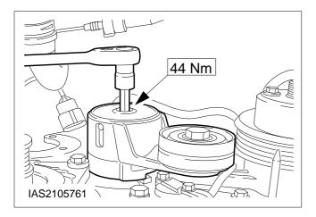
102. Fit the bracket for the alternator/power steering pump.
