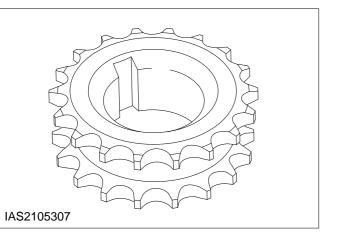
**NOTE:** The chamfer points away from the cylinder block.
