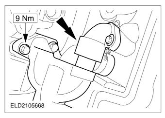
94. Fit the cylinder head covers (left-hand side shown).
