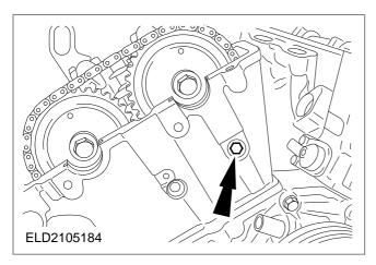
43. Remove the PCV bracket and disconnect the fuel lines.
