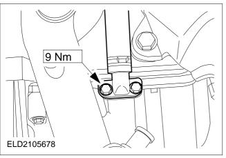
76. Fit the PCV connector (right-hand side shown).
