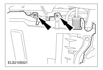
4. Remove the nuts from the shroud for the radiator fan.
