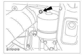
8. Remove the lower exhaust manifold nut from the catalytic converter.
