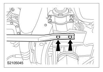
7. Detach the transverse brace from the front crossmember (left-hand side shown).
