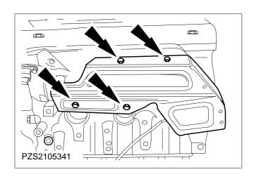
5. Remove the right-hand heat shield (left-hand side shown).
