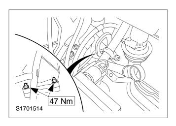
17. Screw the upper exhaust manifold nuts onto the catalytic converter.
