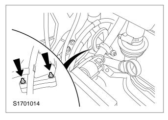
6. Remove the upper exhaust manifold bolts from the catalytic converter.
