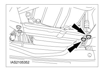
9. Detach the right-hand catalytic converter from the bracket.
