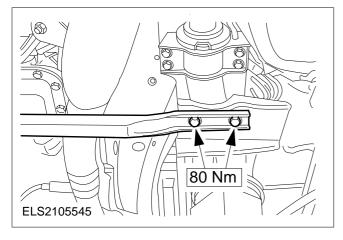
16. Attach the transverse brace to the front crossmember (left-hand side shown).
