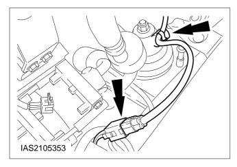
10. Disconnect the HO2S multiplugs and detach them from the engine mounting (left-hand side shown).
