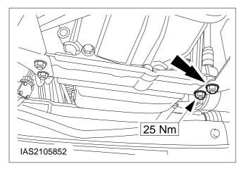
14. Fit the right-hand catalytic converter to the bracket.
