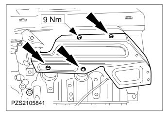
18. Fit the right-hand heat shield (left-hand side shown).
