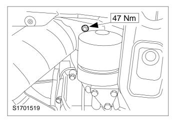
15. Fit the lower exhaust manifold nut to the catalytic converter.
