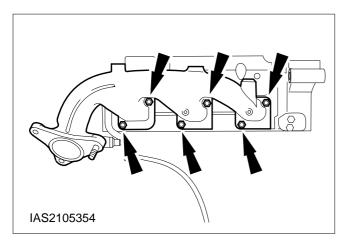
11. Remove the exhaust manifold.
