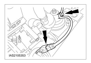
13. Connect the HO2S multiplugs and attach them to the engine mounting (left-hand side shown).
