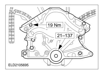
**NOTE:** The left-hand chain guides are attached to the timing chain housing.
