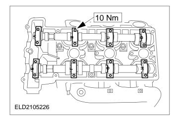
**NOTE:** The wider contact areas of camshaft bearing caps 1 and 5 and A and E point towards the middle.
