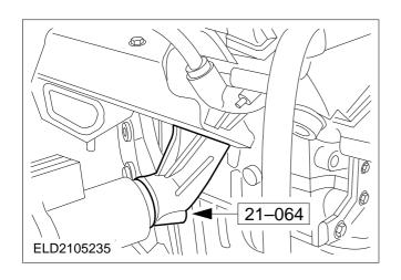
122. Detach the engine from the assembly stand.
