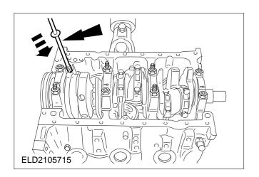
65. Fit the oil pump drive shaft in the hexagonal drive.
