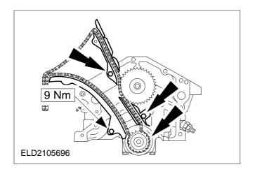
70. Fit the pressure pad of the oil pump drive bearing housing.
