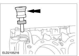
66. Fit the oil pump and oil baffle.
