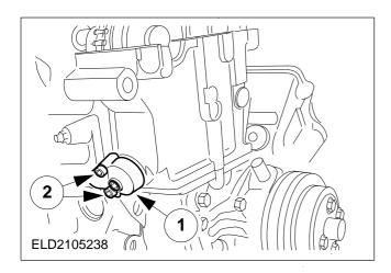
**NOTE:** The chain tensioner is locked once there is an audible click and when it has reached its stop.
