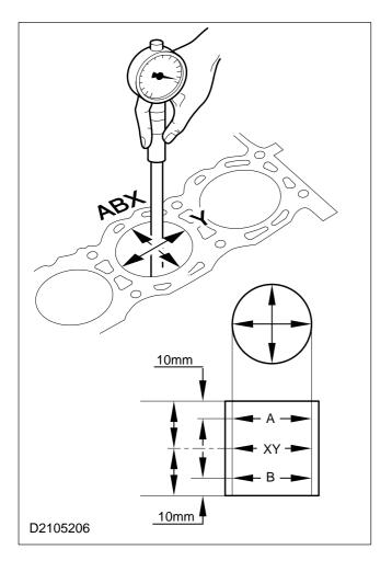
Measure the cylinder bores 48. Measure the cylinder bores.
