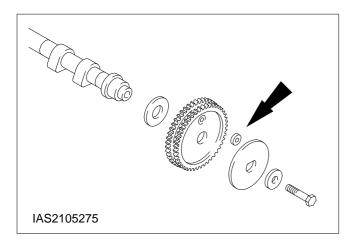
**NOTE:** The drive plate follower must engage in the bore on the camshaft sprocket.
