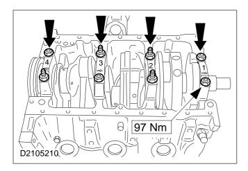
**NOTE:** Installation position of the studs.
