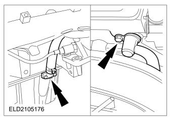
17. Remove the exhaust manifold heat shields (left-hand side shown).
