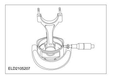
Measure the pistons and piston rings. 49. Measure the pistons.
