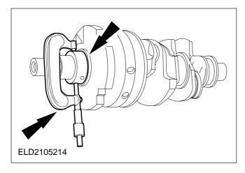
**NOTE:** Measure the clearance with the ring protruding from the groove.
