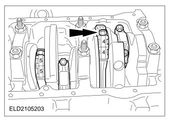
41. Remove the bearing plate and withdraw the intermediate shaft.
