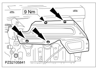
103. Fit the PCV connector (left-hand side shown).
