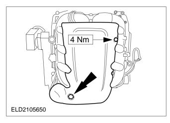
118. Fit the ignition coil bracket.
