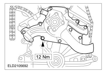
**NOTE:** Tightening sequence and different bolt lengths.
